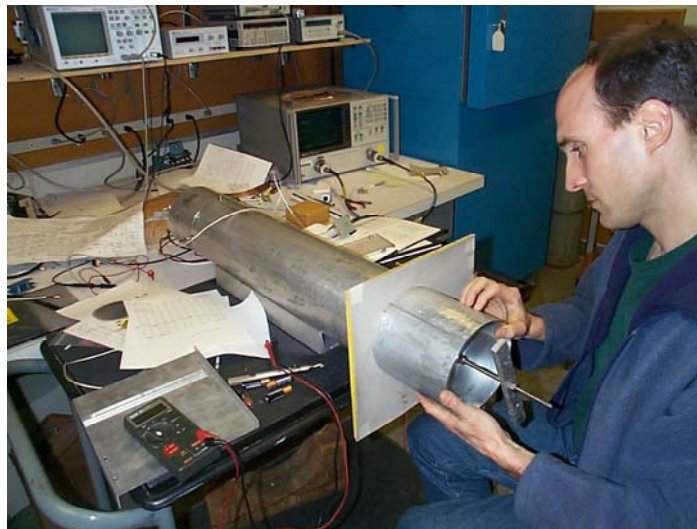
Figure 7. Transmission test setup with the backshort installed.
